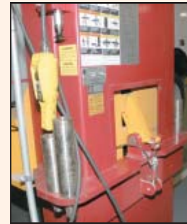
▲ Mohawk's all position mechanical and hydraulic safety systems lock the vehicles at ALL working heights. Mohawk safeties consist of 1 1/2" plate steel locks engaging into the slotted carriage lock racks every 6" inches.
