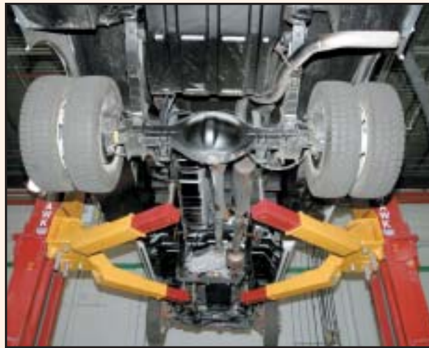
▲ Mohawk's TP-26, TP-30 gives FULL under vehicle access for all repairs, yet takes up minimal bay space, while leaving the wheels hanging free for tire, brake or any other necessary repairs.
