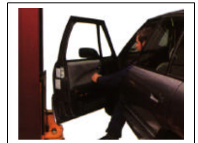
Asymmetric design not required as 10' inside clearance leaves plenty of room for damage-free door openings
