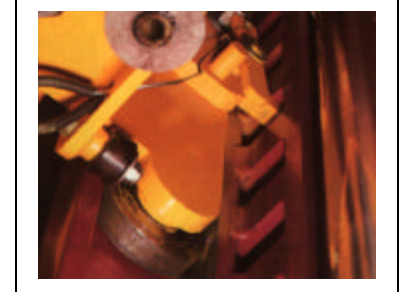
All position mechanical locks in both columns the full length of travel.
